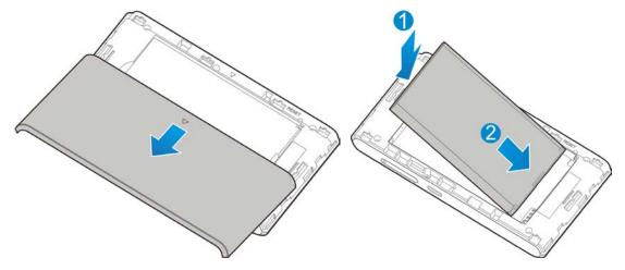
2. Place the battery cover over the battery compartment and press it downward until it clicks into place.
