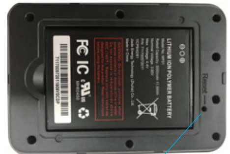
Factory Reset Pinhole
